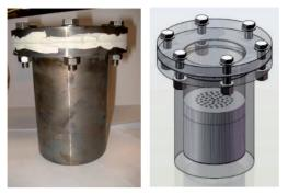
Figure VI: Sealing reactor II of special steel to support 9.8 bars at 1000°C.
